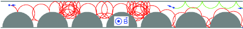
Figure 4: Electrons move under the influence of a perpendicular magnetic field in a structure which is designed to allow for the simultaneous presence of ballistic and diffusive transport. The characteristic feature is that backscattering of electrons occurs only at one of the two boundaries of the channel. A periodic arrangement of large semicircular obstacles is shown here for clarity, but it could be replaced, e.g., by a boundary with a rough surface [5].
