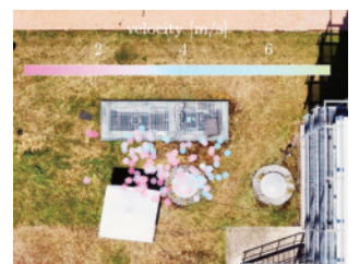
Figure 2.18: Velocity measured from helium filled soap bubbles at the MPI-DS.
