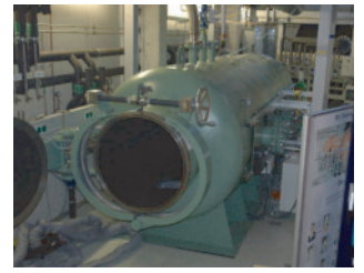
Figure 9.19: The “Cigar”, a general-purpose pressure vessel
