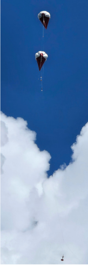
Figure 5.20: The MPCK during the IMPACT field campaign, May–June 2024. Several instruments can be seen on the line, including a WinDart at the bottom right of the picture.
