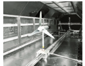
Figure 2.17: Experiments with a model in the VDTT.
