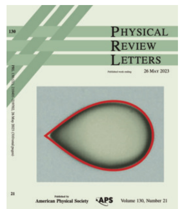
Figure 4.12: Experimental snapshot of an originally spherical, water-emersed silicon droplet which was engulfed by a slowly moving freezing front (0.2 \mu\text{m/s} ). This leads to droplet deformation, due to the competition of thermal Marangoni forces and disjoining pressure in the lubrication layer around the droplet. The red curve is from our theory, showing a perfect match with the experiments. Figure taken from [7] and the Cover of that PRL issue.
