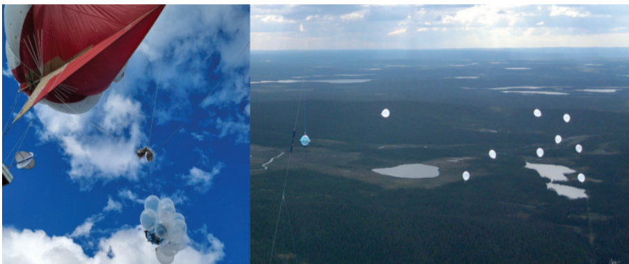
Figure 5.25: Left: Set of balloons attached to the CloudKite before a flight. Right: Release of balloons from an altitude of 600 m above ground level.
