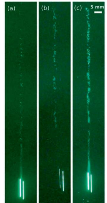
**Figure 6.32:** Nucleation of water droplets and ice particles in the wake of a falling drop (diameter  $\sim 2$  mm) that is warm relative to the ambient cold conditions. Ambient temperature  $\sim -18$  °C, relative humidity  $\sim 60$  %. The initial drop temperatures are (a) 10 °C, (b) 10 °C, and (c) 20 °C. The number concentration of the Snomax aerosol particles in the chamber was  $\sim 10^4$  cm $^{-3}$  in all cases except in (a), where it was  $\sim 10^3$  cm $^{-3}$ .
