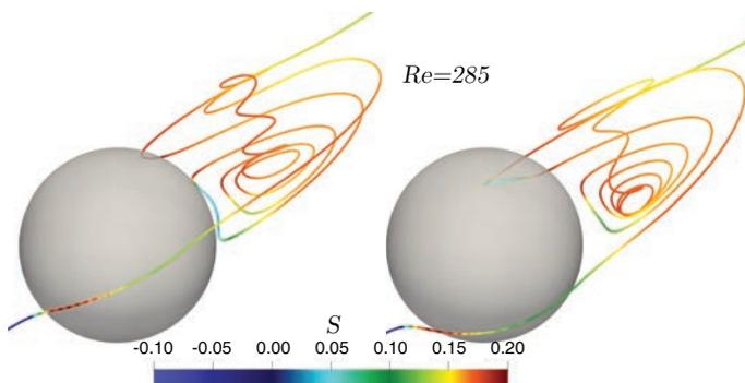
**Figure 6.33:** Tracks of the excess water vapour ( $S > 0$ ) that two aerosols experience when they entered the water vapour rich environment behind a precipitating frozen hydrometeor at 0 °C temperature falling through an ambient at  $-15$  °C and 95% relative humidity condition.
