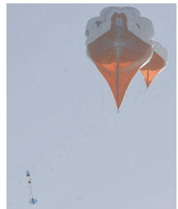
**Figure 6.29:** The 250 m<sup>3</sup> MPCK flying with a 35 m<sup>3</sup> aerostat flying in tandem for more lift from the [RV Maria S. Merian](#) as part of the [EUREC<sup>4</sup>A](#) campaign. The instrument package is hanging on the line in the bottom left of the photo.
