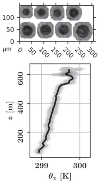
**Figure 6.30:** (Top) Hologram reconstruction of large cloud droplets. (Bottom) vertical profile of the virtual potential temperature  $\theta_v$  from a fast ascent (grey points are ind. measurements and black line is the 15 m average).
