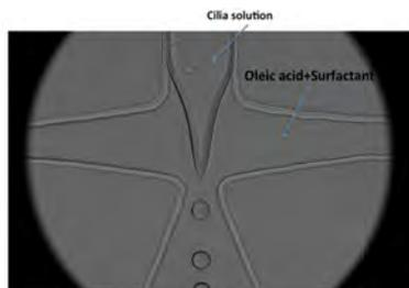
Figure 3.6: Encapsulation of isolated cilia inside droplets generated in a microfluidic setup.
