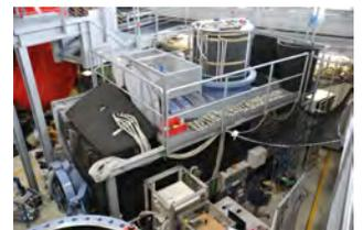
The “U-Boot”, a general-purpose pressure vessel, housing the High-Pressure Convection Facility (HPCF)
